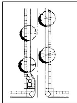
Figure 5.9 - curb projections or “bulb-out.”
