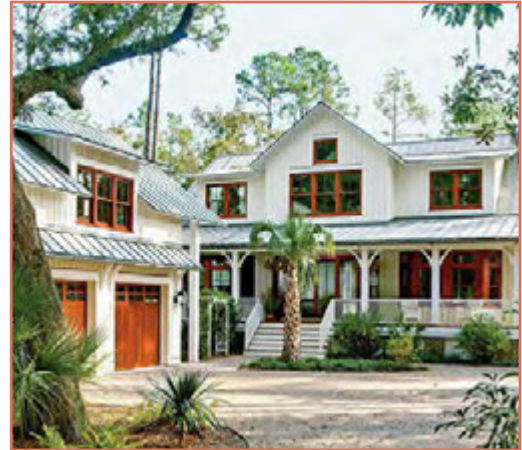
Garages should not dominate the streetscape. Front-loaded garages should be located to the rear, side-loaded, or recessed from the front facade
