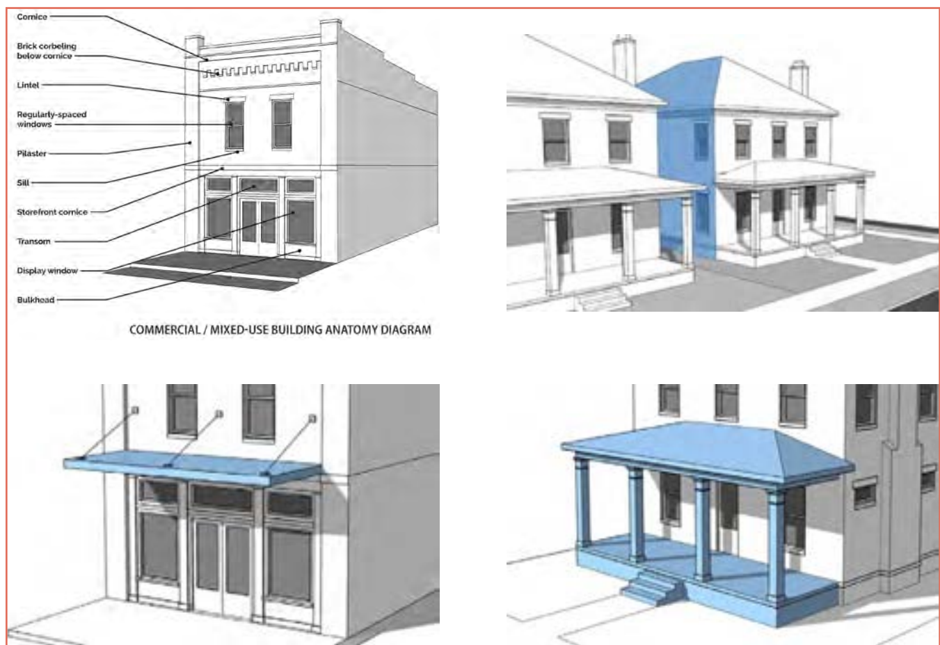
Sample Design Guidelines - Graphics from Fayetteville, NC Source: The Walker Collaborative / Common Ground Urban Design + Planning
