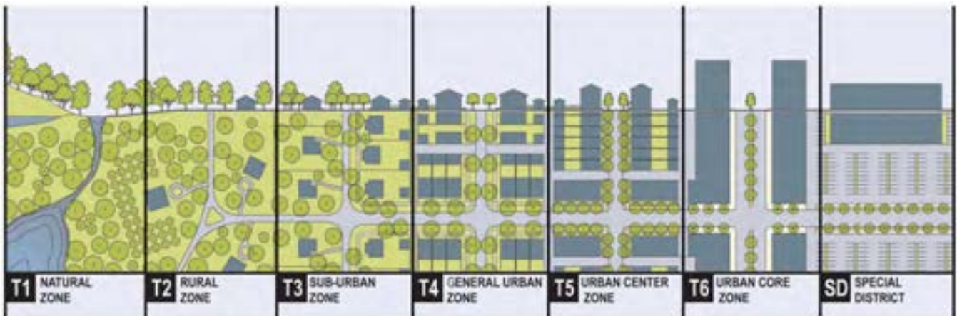
The diagram above illustrates the concept of the transect. The transect is a "system that identifies the varieties of human and natural habitats by intensity and mix, both for analysis and to project future urbanism through codes." (from The Lexicon of New Urbanism by Duany Plater-Zyberk & Company) The rural to urban transect is divided into six zones and a special designation (areas that do not fit within one of the other zones) for application to the different contexts within plans and codes. Each zone varies in its physical character and intensity based on the typical contexts of human settlement from rural to urban.
