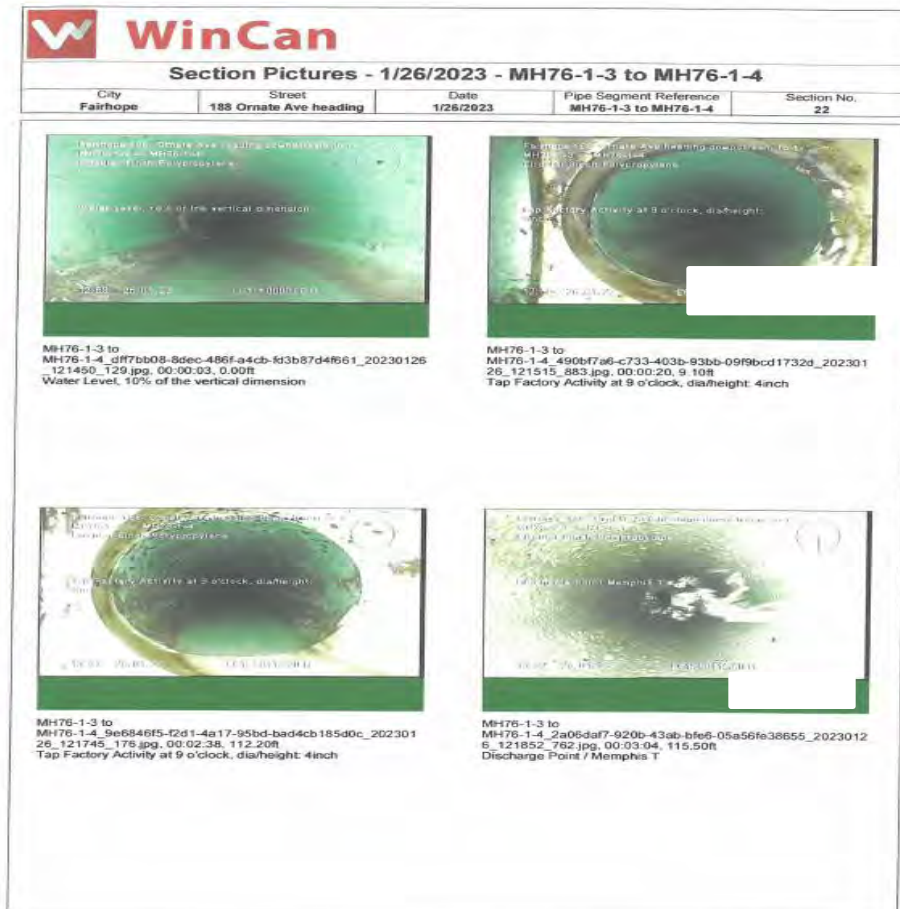
Example of Sewer Line Video from 2023 to check for infiltrations into stormwater systems.
