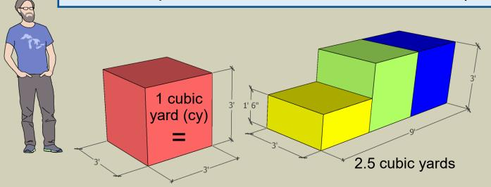
The bed of a full size standard pickup has dimensions of: 8' long X 5.33' wide X 1.5' high. When loaded level full, a truck of this size will hold 2.5 cubic yards of material.
