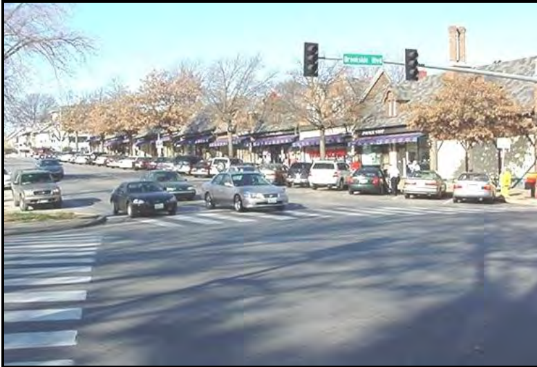
Street function / street design Village center at the intersection of two arterial streets, using angled and parallel parking and “bulb-outs” for pedestrian crossing.
