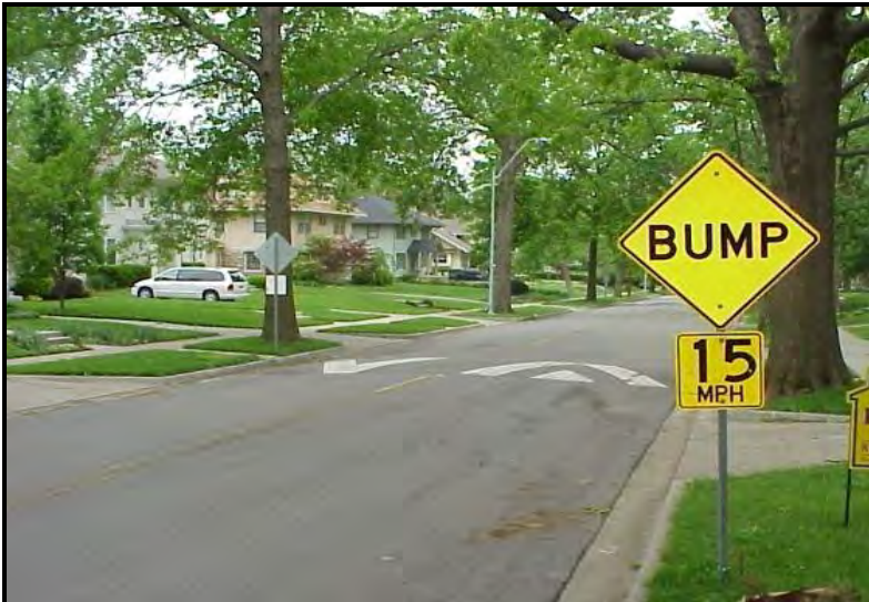
Traffic calming – Speed hump on collector street with residential uses fronting on street.
