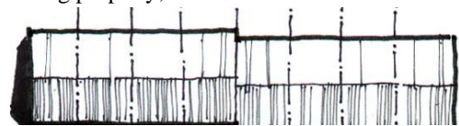
Figure 3-1. Townhouse units of more than 4 shall have a differentiated front building line of at least 4 feet and no single building shall have more than 8 units.
