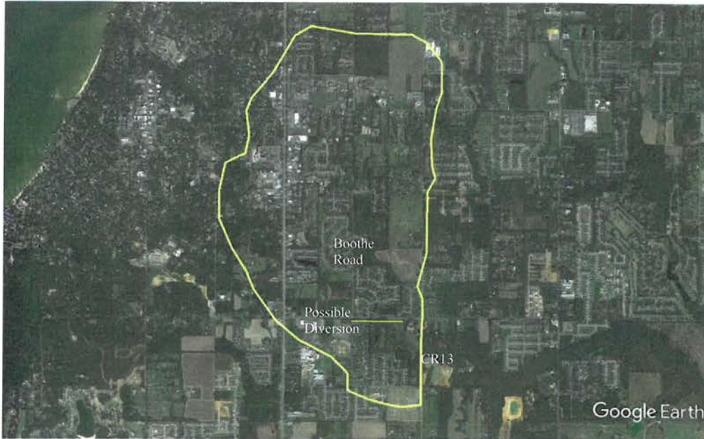
Figure 2. Approximate drainage area to downstream of Twin Beech Road at CR13 and possible structure location
