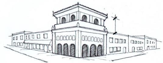
Figure 6-15. Height deviations buildings along a single block should be small except that taller buildings may anchor corners of blocks.
