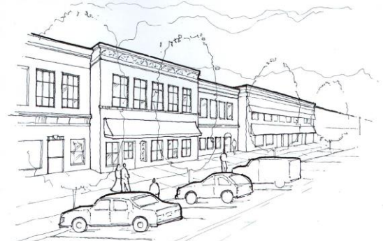
Figure 6-14. Long building facades should use variations in building mass while still presenting a consistent streetscape.
