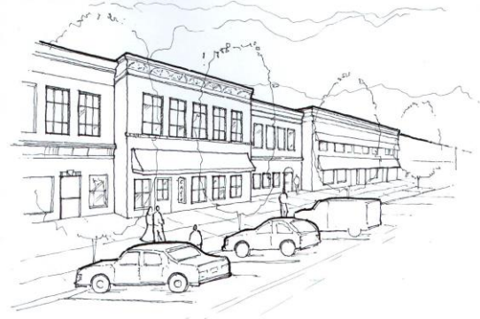
Figure 6-25. Long building facades should use variations in building mass while still presenting a consistent streetscape.
