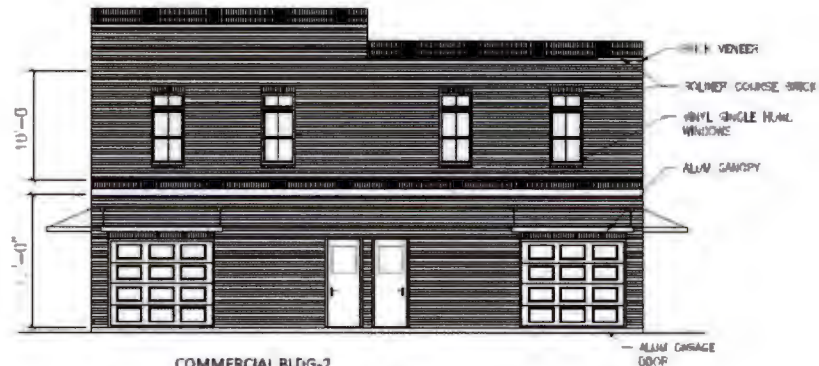
G A-201 COMMERCIAL BLDG-2 SIDE VIEW SCALE: 1/8"=1'-0"
