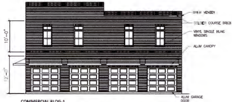
E A-201 COMMERCIAL BLDG-1 SIDE VIEW SCALE: 1/8"=1'-0"
