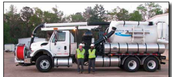
(L to R): Josh Hughes and Reggie Ford are shown with the 2012 Vactor 2100 Plus Truck, which is the latest addition to Dothan Utilities' sanitary sewer cleaning fleet.
