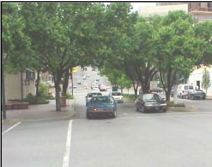
Traffic calming - Arterial street with center median.
